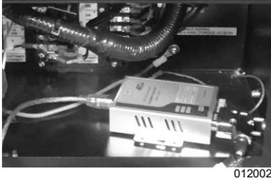
**Figure 3-8. USB Converter Mounted on Interior Base**
